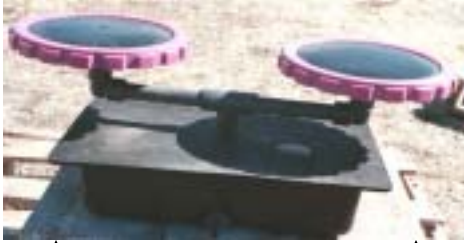
↑ Diffuser pads on aerator 9/12/03 Photo by Bob Bates ↑
